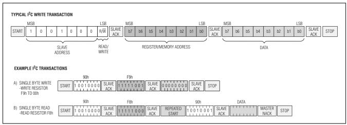
Figure 2. I<sup>2</sup>C Communication Examples
