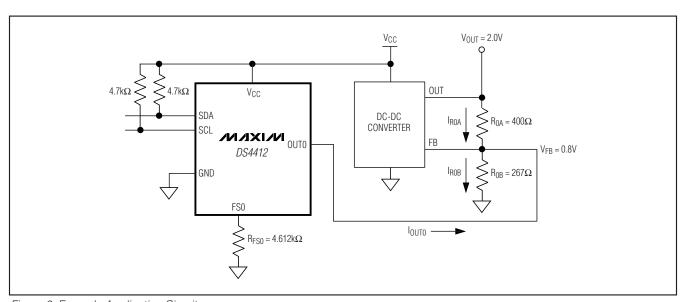
Figure 3. Example Application Circuit
