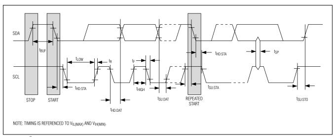
Figure 1. I<sup>2</sup>C Timing Diagram
